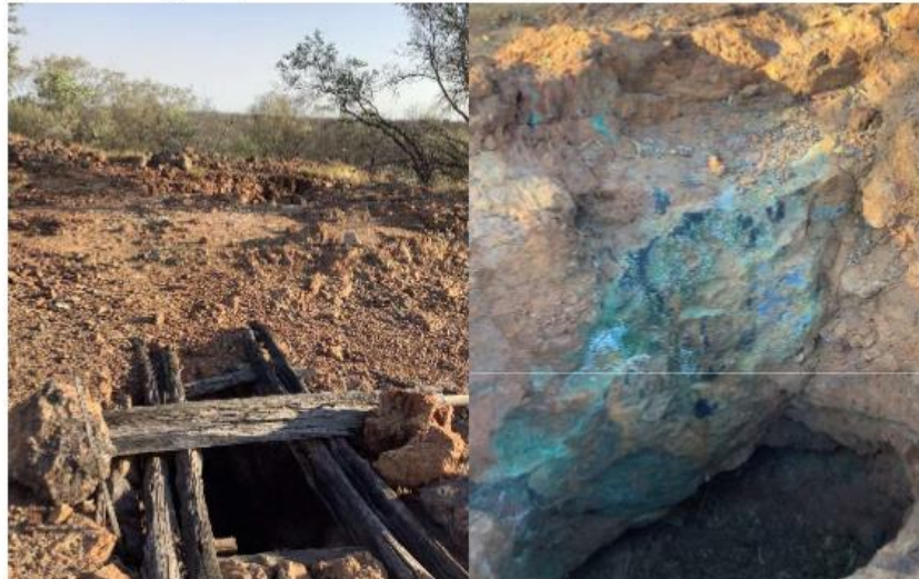
Figure 6-6. Silver King workings: Shaft and trench (LHS), shallow pit with copper oxide minerals (RHS).
